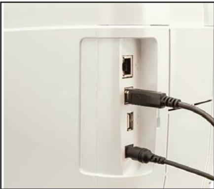
Interface for USB (high speed), built in 10/100 ethernet, Wi-Fi (optional)
